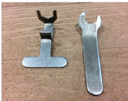
The kit came with the wrench seen on the left, but the author felt that two types were needed for various installations so he reached into his toolbox and modified the one on the right.
