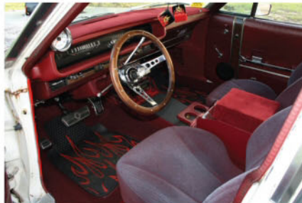
James replaced the original front bench seat on the '68 with a set of bucket seats from an estate sale. The rear seat and its original upholstery were retained.
