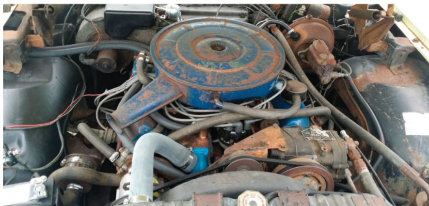
The two-barrel version of the 390 was new for 1967 and was rated at 270 horsepower at 4400 rpm. Note the optional air conditioning and power brakes.
