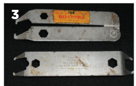
While not new and shiny, these are two handy tools for removing windshield wiper arms.
