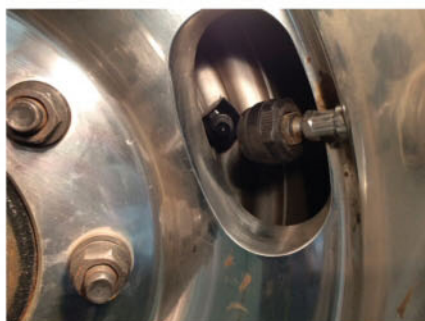
Here you can see the flow-through and anti-theft sensors installed on a dual-rim setup. The kit can be ordered with a mixture of these types of sensors.
