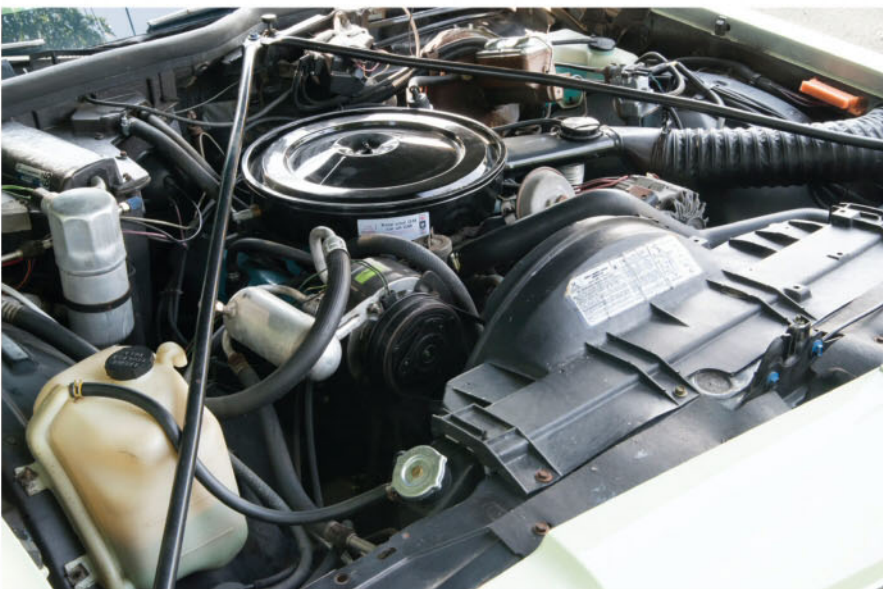
Emissions equipment was growing increasingly complex by 1979, but the 403 is still visible.
