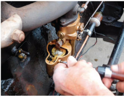
The Marvel carburetor's float had to be adjusted at the Kwik-Trip.
