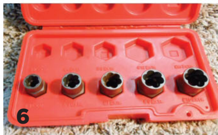
6 Here is a special socket set for removing rounded, damaged nuts and bolts.
