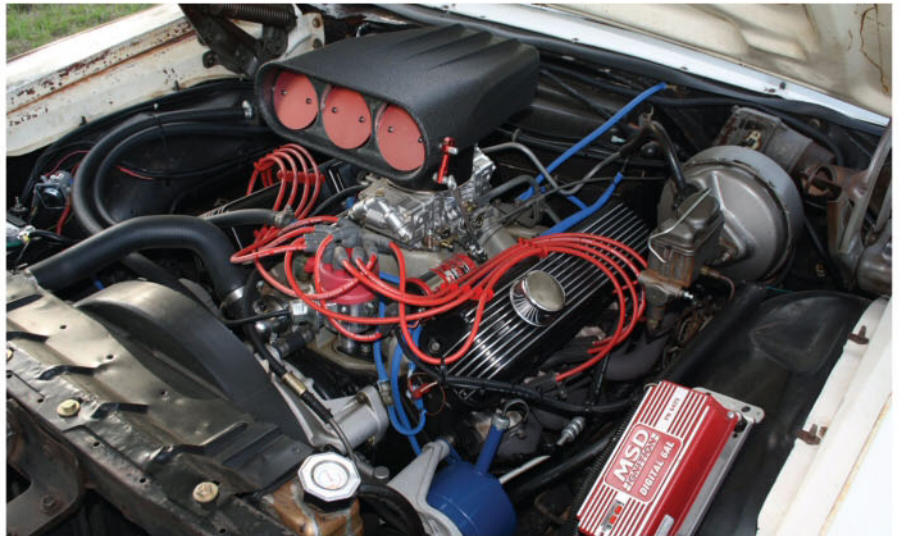
The original Y-code 390 2-bbl. was rebuilt including a .030 overbore and a Holley 770 Street Avenger four-venturi carburetor. James cut a hole in the hood to give clearance for the air intake mounted atop the carburetor.
