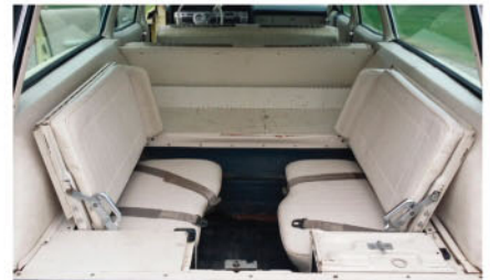
The dual-facing rear seats made this Country Squire a nine-passenger model. When not in use they could be folded down for additional cargo space.
