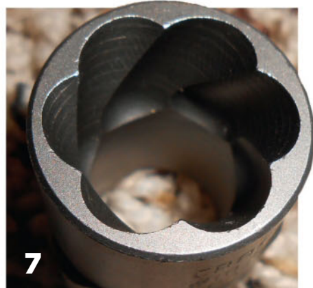
7 This socket is designed for removing right-hand thread only.
