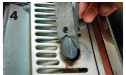
The tool is used to overcome spring pressure and make arm removal easy and damage-free.
