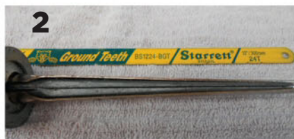
The nose of the tool has a tapered conical shape that wedges the blade securely into place.
