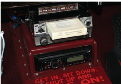
An aftermarket, period-correct 8-track stereo (with a Ford-issued 8-track tape) is suspended from the dash and a modern CD player is mounted in a console custom-built by the owner. The optional “Convenience Group” is visible above the stereo equipment.
