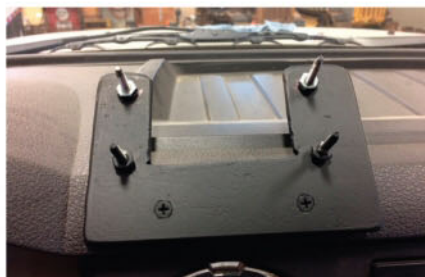
The author wasn't satisfied with the mounting options provided with the kit, so he made his own bracket.
